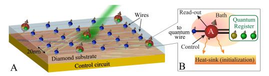
**Diamond-based quantum computing architecture**: A) The NV center (actuator) in each register is addressed optically. Nitrogen spins qubit wires connect the registers. The diamond rests atop a nano-fabricated circuit that provides static magnetic fields and microwave control. B) Quantum registers comprise an actuator and nearby nuclear spins that are strongly coupled to the actuator but interact weakly with the bath, thus providing long coherence times.
